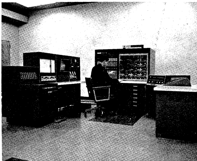
Figure 17—680 10V computer with display wing
